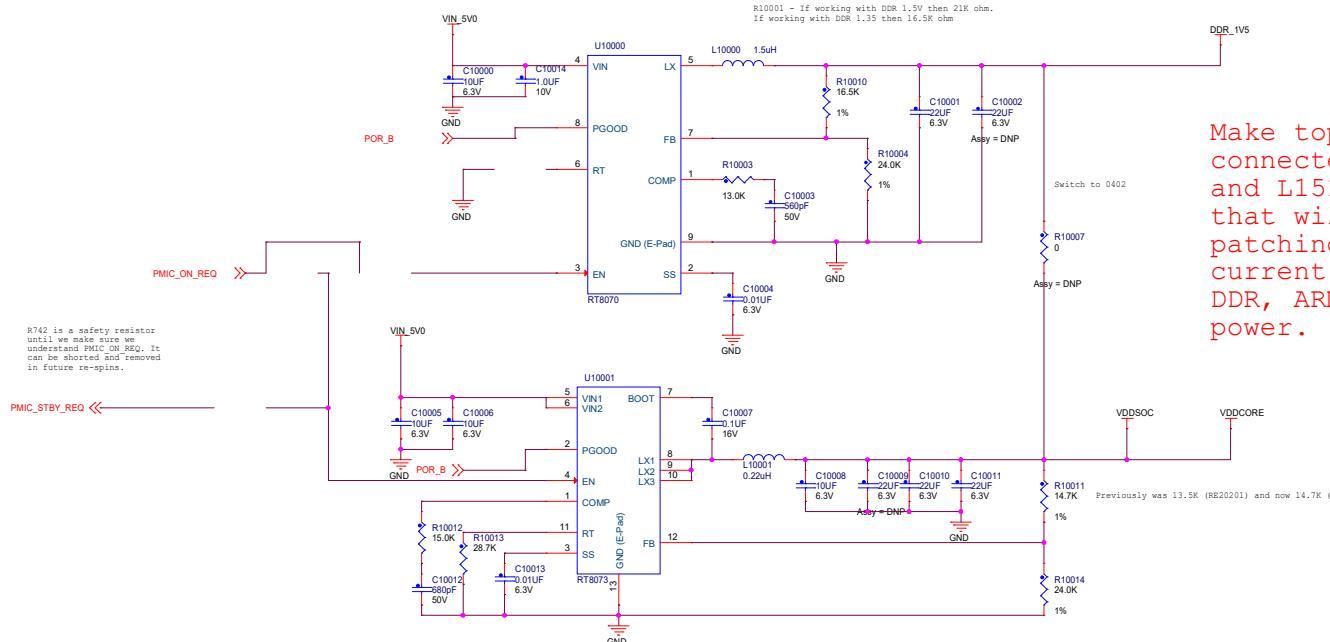
Make top layer planes connected to L1514 and L1515 in a way that will enable patching a board for current sensing or DDR, ARM and SOC power.
